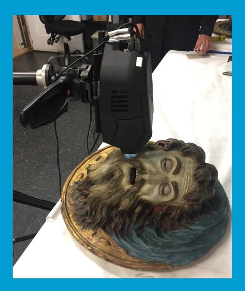
Figure 3. In situ analysis of Roldán's *Head of* Saint Paul by means of X-ray fluorescence spectroscopy.
