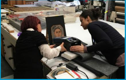
Figure 3. NICS scientists Federica Pozzi and Elena Basso take in situ Raman measurements of selected areas of a portrait using a handheld Raman spectrometer.
