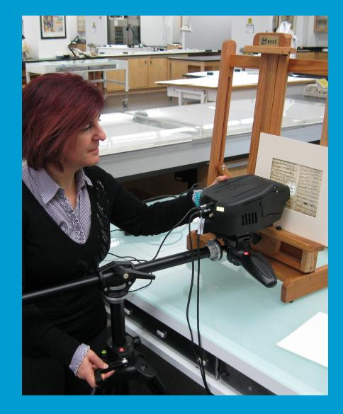
Figure 1. NICS scientist Elena Basso sets up a portable X-ray fluorescence spectrometer for in situ analysis of one of the manuscripts.
