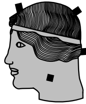
2. Wax model over core with protruding chaplets.
