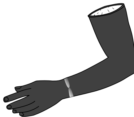
10. Hand joined to arm by flow weld.
