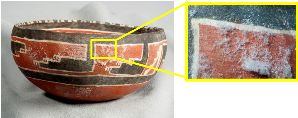
Figure 3. Acids and bases from low VOC case construction materials reacted to form crystals on a ceramic object housed in a modern display case 2
