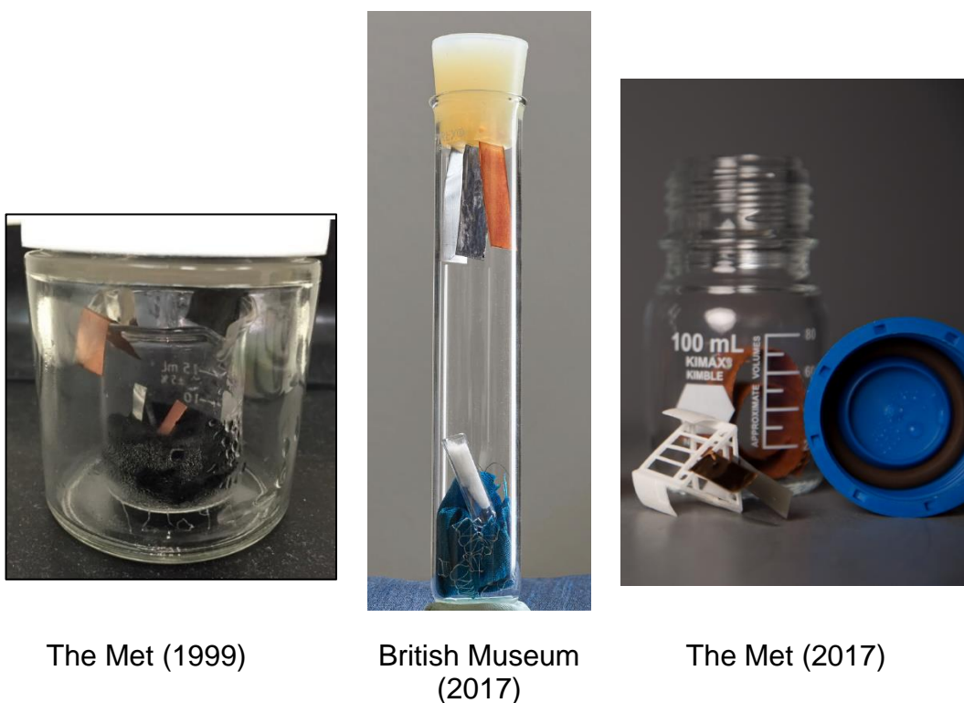
Figure 2. Example Oddy test configurations from The Met 10,11,12 and The British Museum 9
