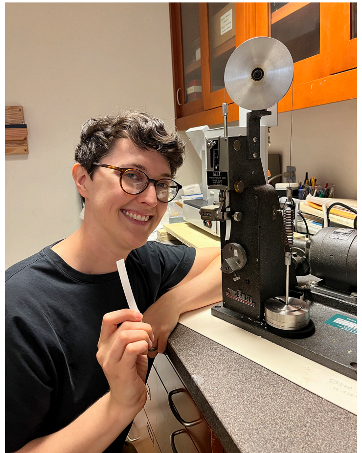
Above: Research Scholar, Cat Stephens, preparing to work with our 1960s MIT- style folding endurance tester. This machine allows the comparison of the relative strengths of different papers. Credit: Katie Sanderson
