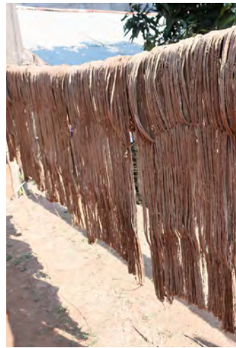
Skeins of yarn drying in the sun. The sun's heat helps the mordant penetrate the cotton fiber
