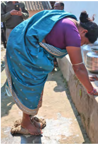
Mordanting of cotton yarn, a difficult fiber to dye. The yarn is soaked in cow-dung paste, then kneaded with the feet
